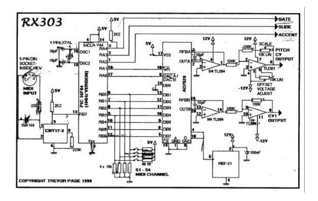
The circuit first receives MIDI messages from a controller and sends them to the CNY17-3 optocoupler. The optocoupler translates the incoming MIDI information to TTL 1's and 0's that the PIC16F84 can understand.
