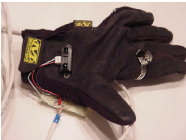
Figure 4: IR Sensor and Underside of Glove
