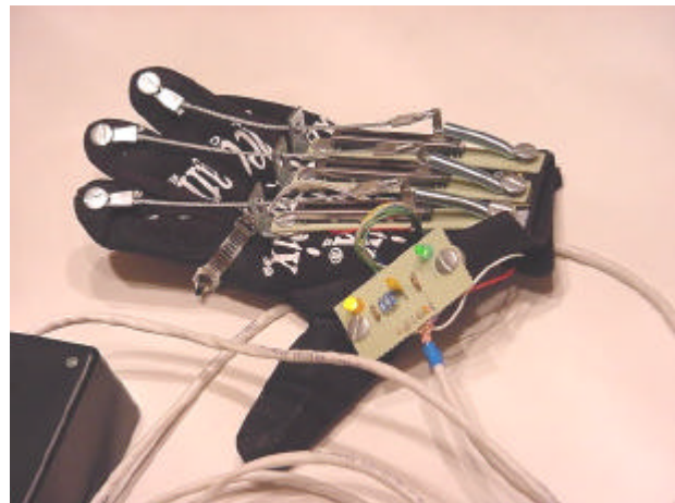
Figure 5: Top of Glove and Cable/Fader Assemblies
