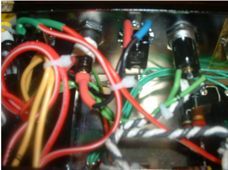
Fig. 2.4 Inner detail of circuit –star ground and filament conductors
