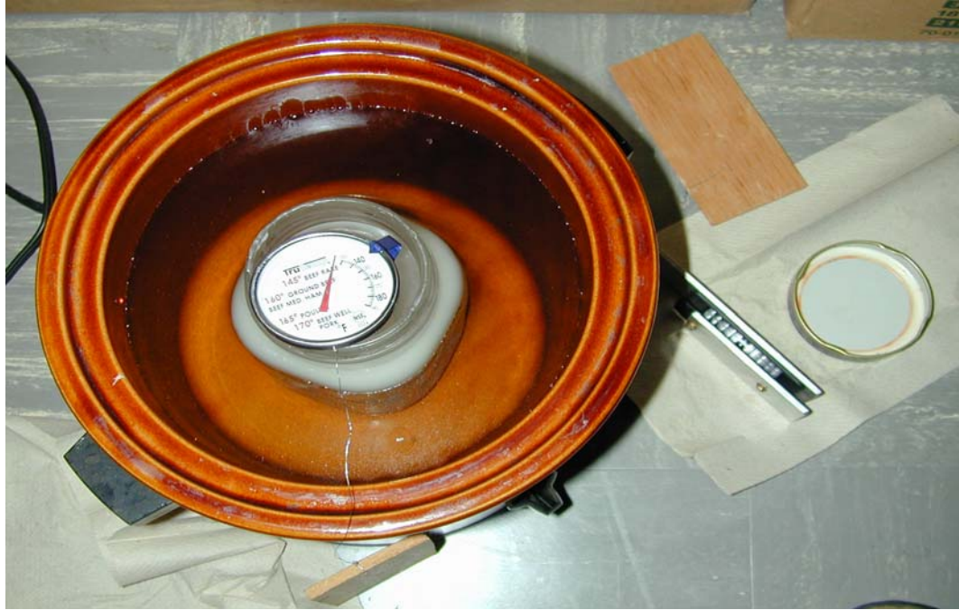
Figure 6. Setup for potting pickups.
