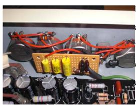
It consists of a lowpass, bandpass, and high pass filters that are controlled by the treble, mid, and bass, respectively. The change in resistance from turning the potentiometers changes the time constant of the RC circuits that are acting as filters and they allow different frequencies through while throwing others away.
