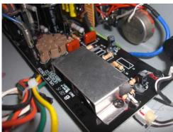
main printed circuit board. To prevent any other interference problems a thin sheet of metal was fashioned in order to cover the tube socket and input. It is grounded by screwing it down with the same screws that hold the printed circuit board in place. I put it in my amp as an extra precaution. It may not be necessary in all cases.
