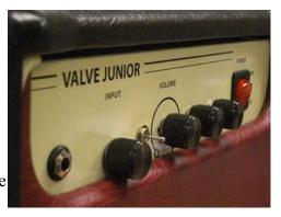
In this tone stack circuit, the potentiometers are used in what is effectively three different filters.
