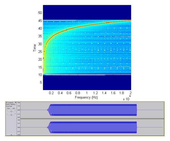
The waveform shows smooth lead-in windowing, and a consistent amplitude. The spectrogram shows very little errant frequencies as the signal sweep smoothly changes frequency. And now, the recorded audition of the above file.
