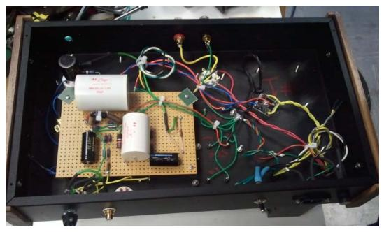
After both of the audio boards and the chasses are complete, they were put together and wired up. I used coax cable for long signal path and input-to-potentiometer signal path, since they are vulnerable to the radiation from the other parts and become sources of 60-cycle hum. Otherwise, I used 22 AWG Belden wire that was provided by the lab.
