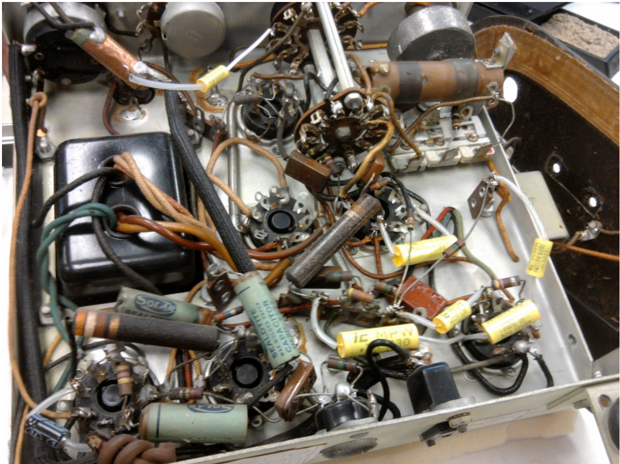
Inside view of 1947 Garod Radio during capacitor replacement
