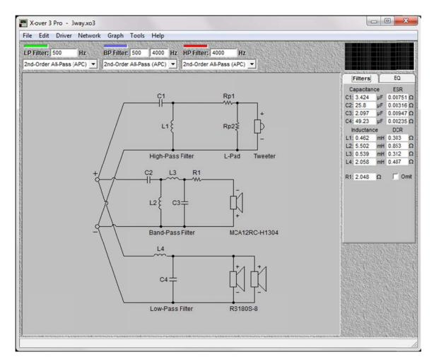
The tweeter high-pass filter contains a resistor network known as an L-pad, which reduces the output of the tweeter by approximately 4 dB. This is necessary because the tweeter is a significantly more efficient driver over the frequency band it is designed to operate in. Without this network, the tweeter would sound louder than the other drivers.
