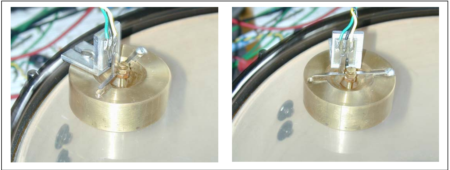
Figure 11: Photographs of the prototype tuner in use. Though the magnets and L iron are off center, the device was successful as a drum tuner. The only real constraint on the device is that the plane in which the magnets sit cannot vary relative to the plane of the Hall probe.
