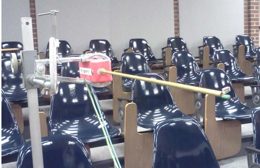
Figure 14 The pressure and particle velocity microphone is placed together, facing towards the speaker in front
