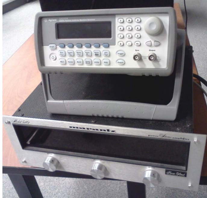
Figure 12 Agilent 33220A Wavefunction generator and a Marantz Model 510 power amplifier used to generate very loud noise.
