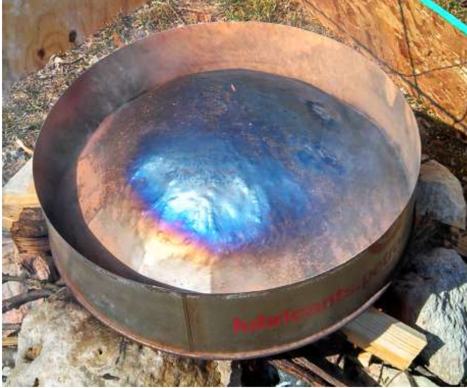
Figure 7: The steel pan being tempered over a wood fire
