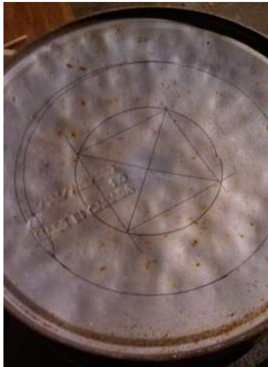
Figure 1: Concentric circles drawn on the bottom of the drum for aiding in the shaping. Photo taken after several blows from the hammer had been delivered
