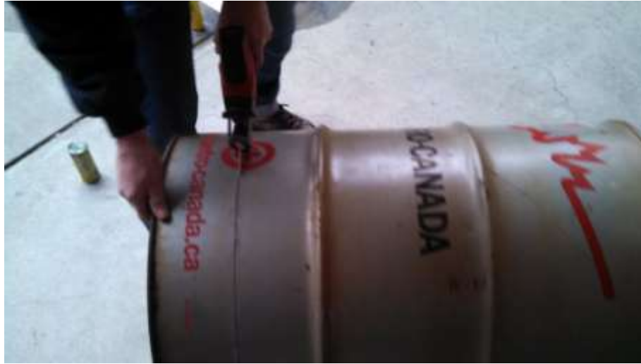
Figure 6: Cutting the drum to the appropriate size
