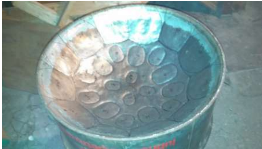
Figure 5: The drum post-grooving
