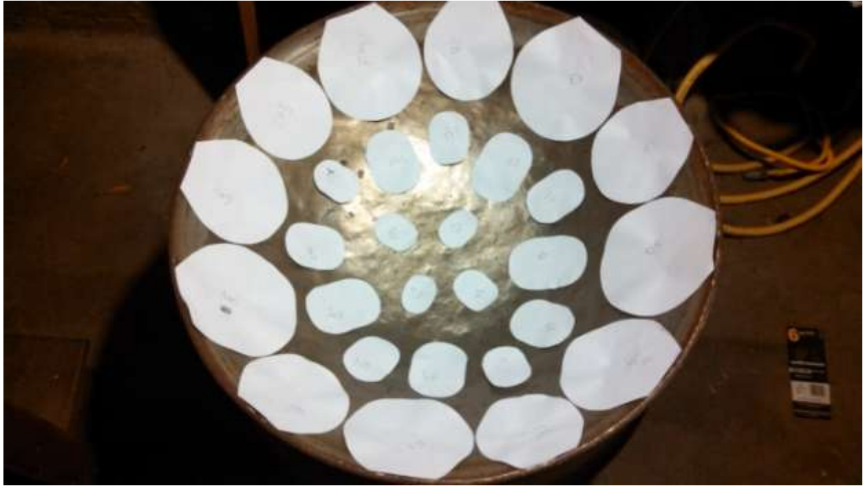
Figure 3: Patterns for the note areas placed on the steel drum
