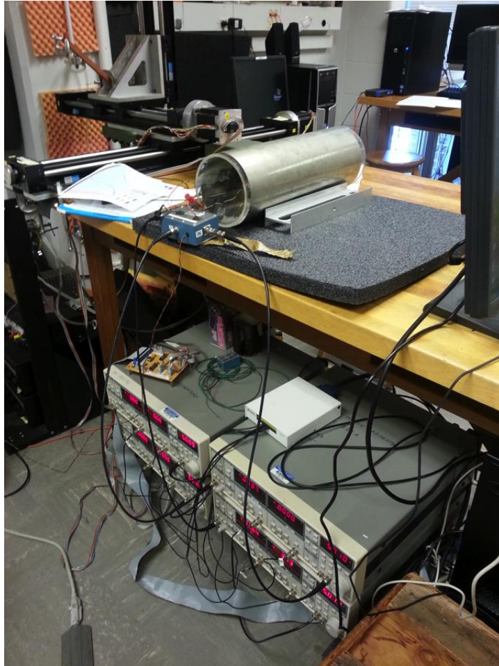
Figure 4: Setup for Measurements, the pickup is placed inside the hole.
