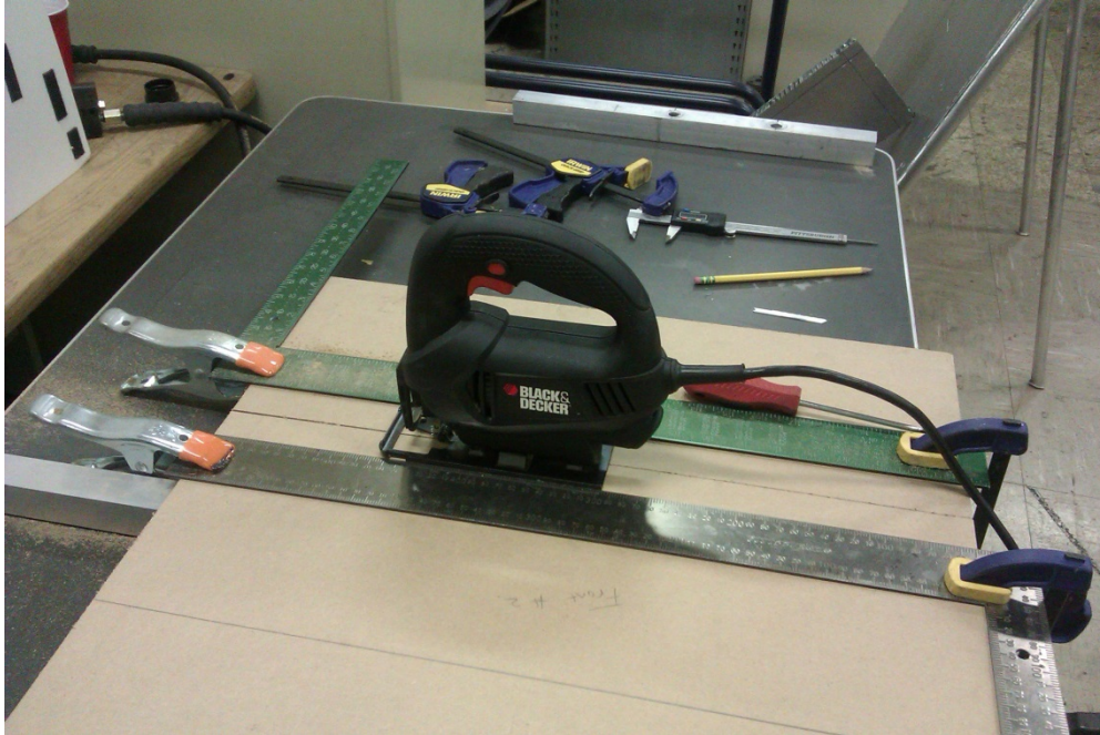
Figure 9: Setup for Cutting the Panels in the MDF
