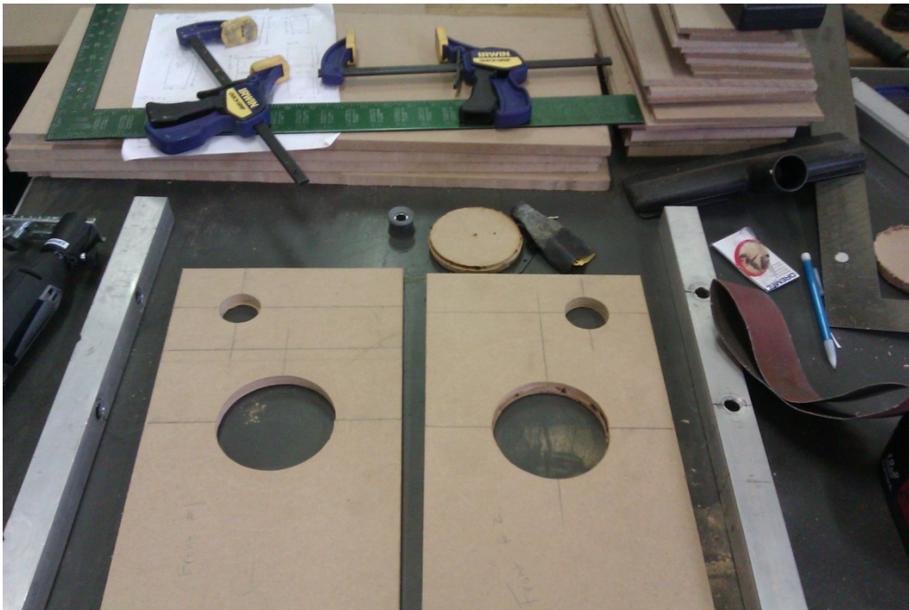
Figure 10: Front Panels Cut out from \frac{1}{2} " MDF
