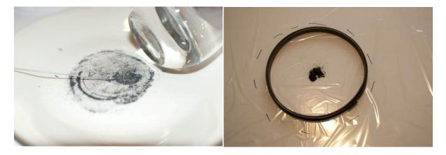
In the finished product, it can be noted that the graphite impregnated Mylar is darker than the untreated:
