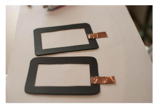
Both pairs of insulator rings were then glued to the Mylar, and allowed to dry:
