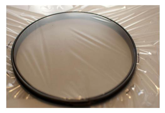
While this does not provide the necessary tension, it begins applying tension to the mylar while the insulating rings are glued on. The Mylar will be heat treated later induce shrinking, and add tension to the system.
