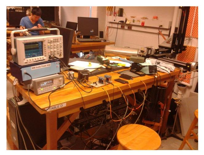
The blue signal on the oscilloscope is the reference signal from the sine wave generator and the yellow is the voltage output from the Edcor audio transformers. Both channels produced audible sound with this setup.
