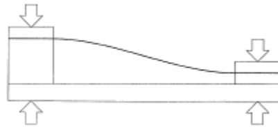
Figure 1: S-shape strip test configuration (Scott & Woodhouse)
