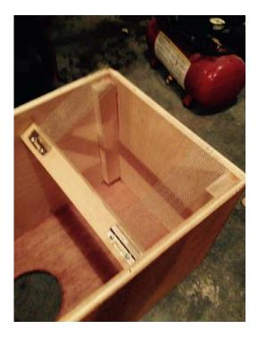
15. Countersink the bottom of the cajon on the edges where the supports are in order to create pilot holes for the rubber feet
