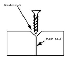
9. Screw in the wood screws into the pilot holes made using the drill
