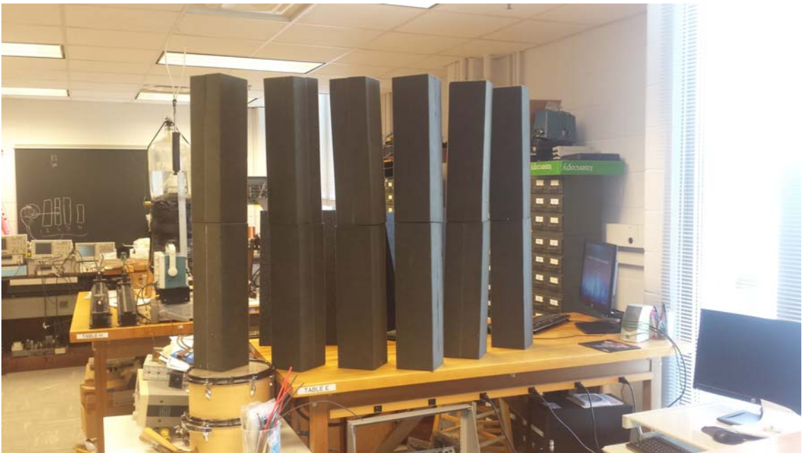
Figure 2: Acoustic padding used to deflect sound waves towards the walls
