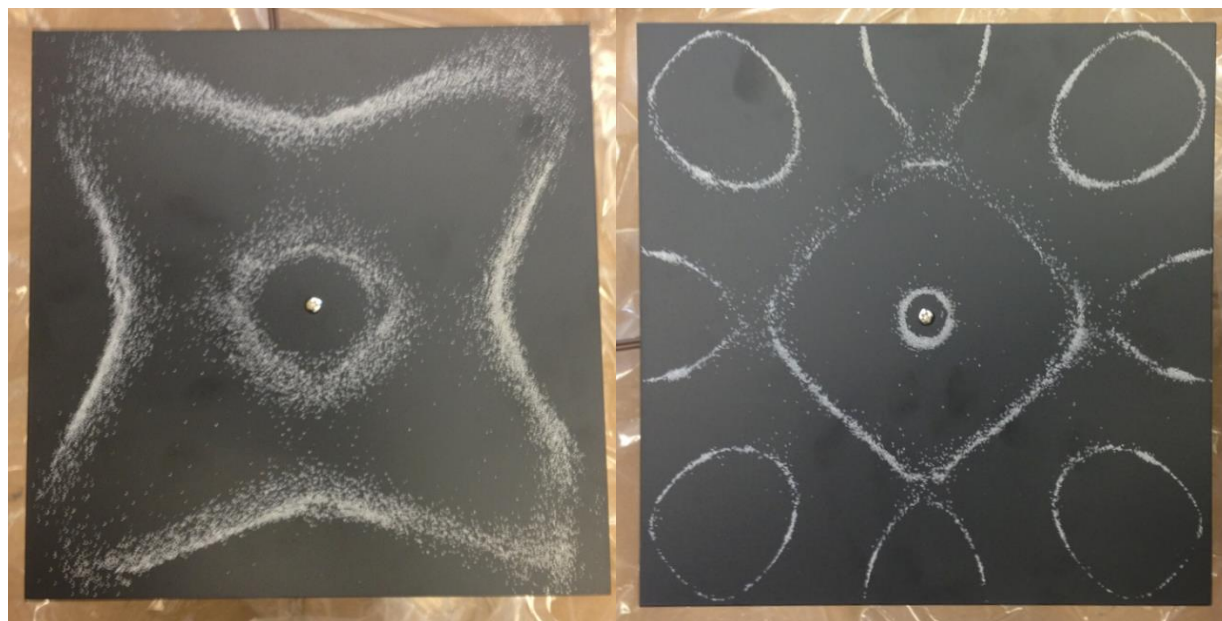
Chladni patterns from the centrally-supported square plate. There is no discernable relation between the patterns produced by the various resonances, except that they all exhibit 4-fold symmetry.
