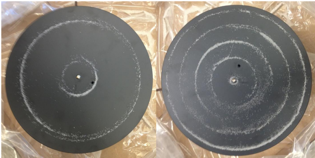
Typical Chladni patterns from a centrally-supported circular plate. Higher frequency resonances contain more circular nodal lines.
