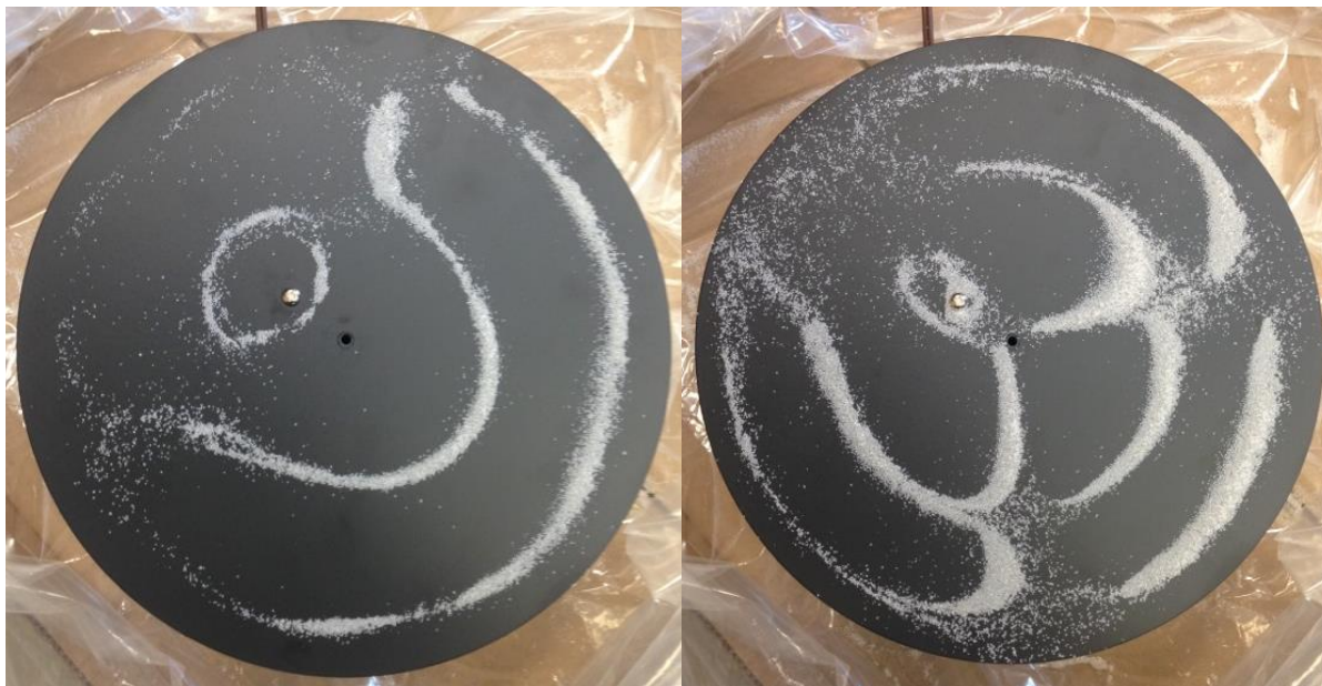
Chladni patterns from the non-centrally-supported circular plate. There is no discernable relation between the patterns produced by the various resonances, except that they all exhibit reflected symmetry.
