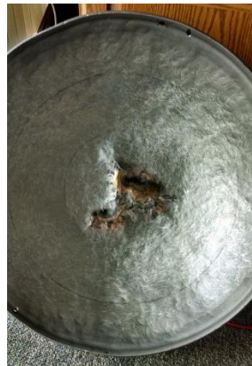
Figure 10. Sanded and welded inner surface of the cut pan.
