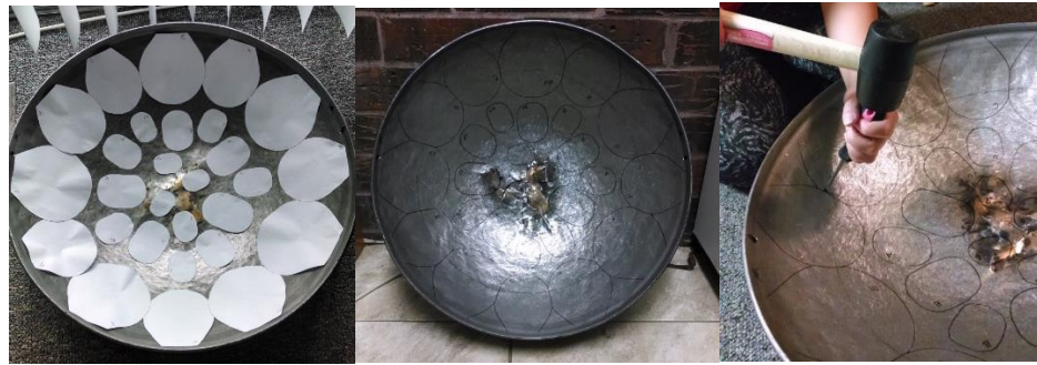
Figure 11. Note templates (left), traced notes (center), and grooving process (right).
