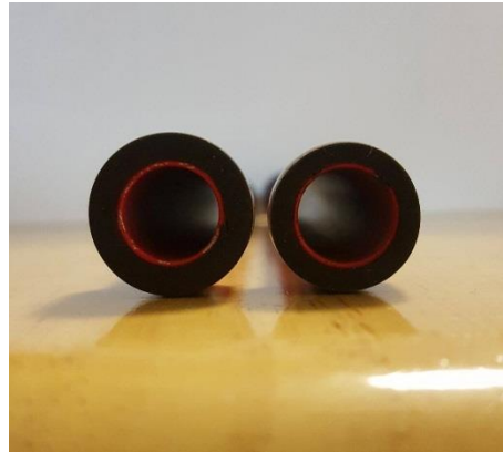
Figure 5. Difference in rubber tip thickness between mallet heads.
