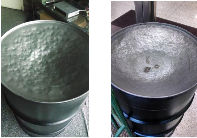
Figure 8. Early in the sinking process (left), compared with the final result (right).
