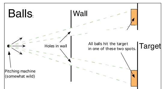
• The flow through two holes is exactly the sum of the flows through each hole separately (so long as they don't bump into each other)
