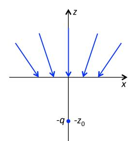
By symmetry (because the charge lies in the z = 0 plane), the field produced at z < 0 (inside the conductor) looks like one produced by a charge -q at  $+z_0$ , i.e., at the same place as the +q charge.
