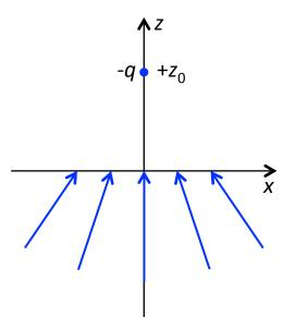
The E fields produced by +q and by the surface charge cancel exactly, leaving E=0 inside the conductor.
