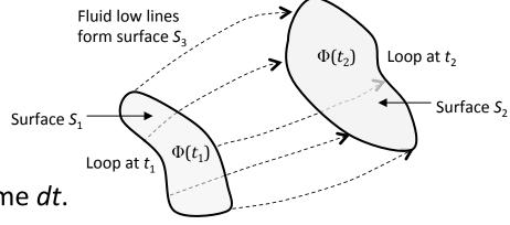
The fluid moves from surface  $S_1$  to  $S_2$  in time dt. We want to calculate:
