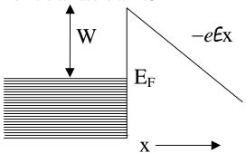
Now an electron at the *Fermi surface* (i.e. with energy  $E_F$ ) can tunnel through the barrier to freedom. In this simple picture, the transmission coefficient for an electron at the
