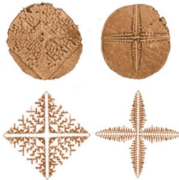
Microphotographic images of pressure-induced dendritic crystals (top row) are remarkably similar to the patterns produced in computer simulations of temperature-driven dendritic crystal growth (bottom row). [1]
