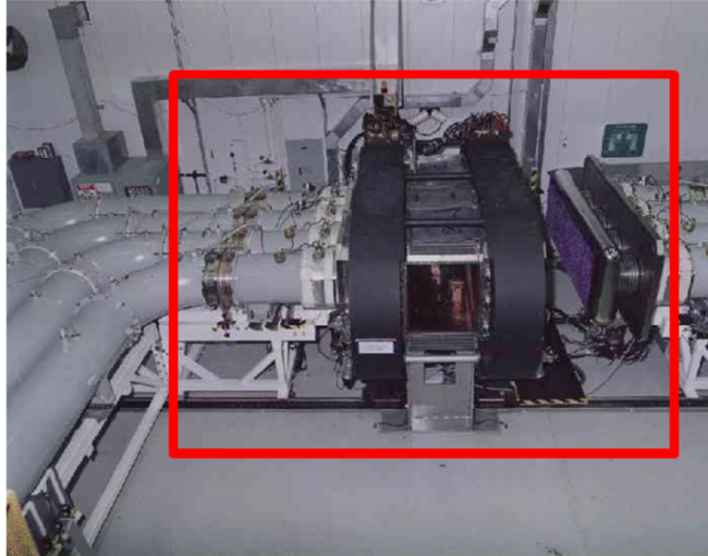
Figure 8. Final amplification stage of the Nike Laser: the 60-cm aperture E-beam-pumped amplifier.
