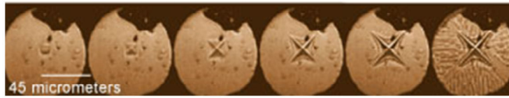
Figure 4. An image sequence from a dDAC experiment shows the growth of a dendritic ice-VI crystal in response to increasing compression. [1]
