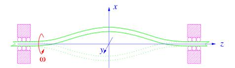
The n = 1 even-parity mode of a whirling shaft.
