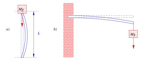
a) Euler's problem: the buckling of a slender column. The rod is used as a column which supports a compressive load Mg directed along the z axis (which is vertical). Show that when the rod buckles slighly (*i.e.* deforms with both ends remaining on the z axis) the total energy, including the gravitational potential energy of the loading mass M, can be approximated by
