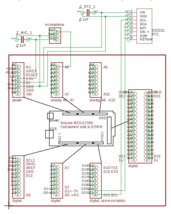
In the circuit, the 0.1µF capacitors serve to reduce possible noise injected into the 3.3V and 5V power supply lines. In general it's a good idea to include a capacitor near each device's power/ground inputs.
