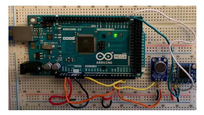
Here's a closeup of the connections to the real time clock. You can see how I make use of the interconnections between the five holes in a column to bring wires from the RTC "breakout board" to the Arduino.
