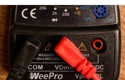
It will probably never come up that you'll want to directly measure a large current by putting the DVM in series with a current source; that's the function of the 10ADC jack into which you could plug the red probe.
