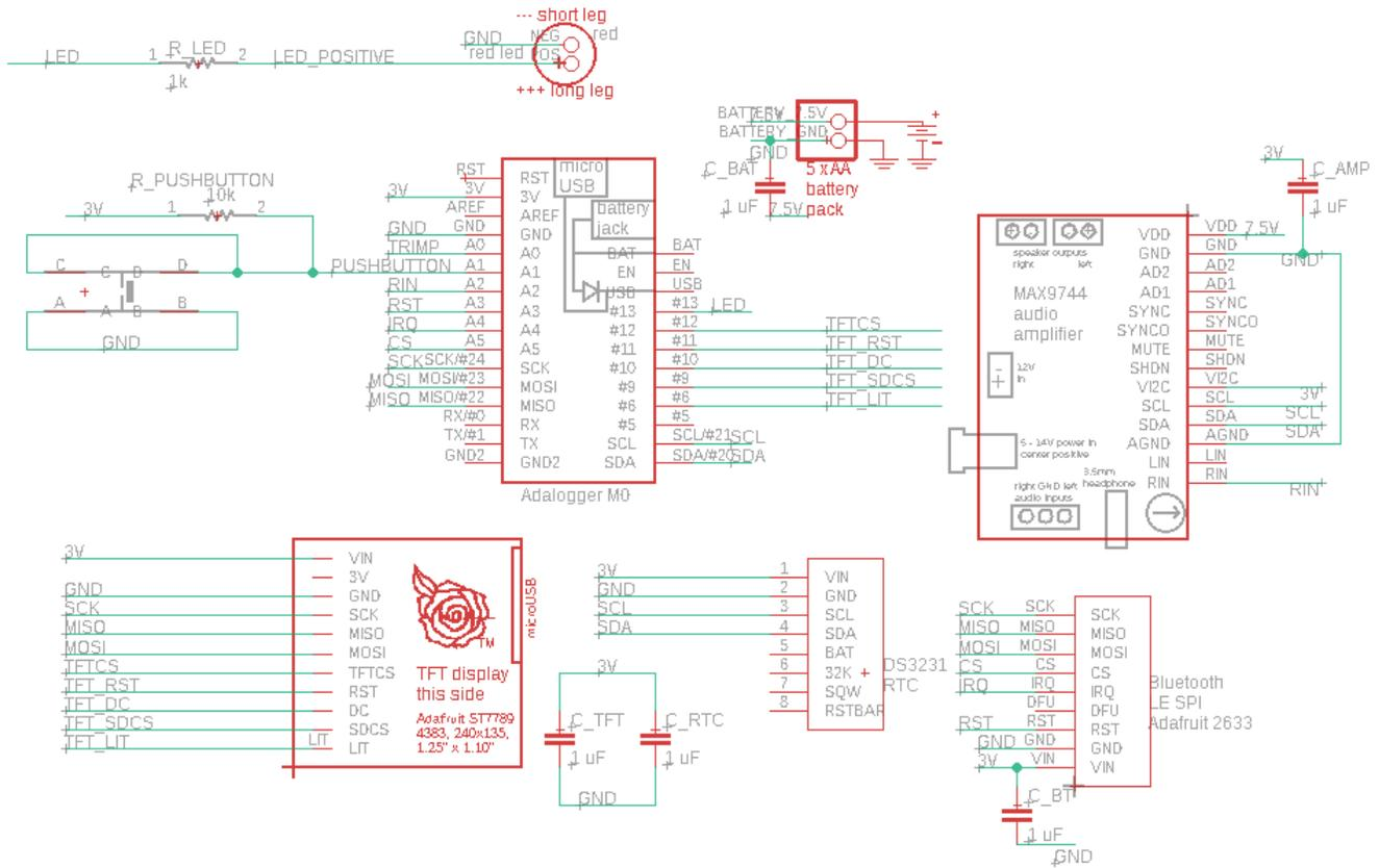
FIG. 14. Schematic of the speaker board.
