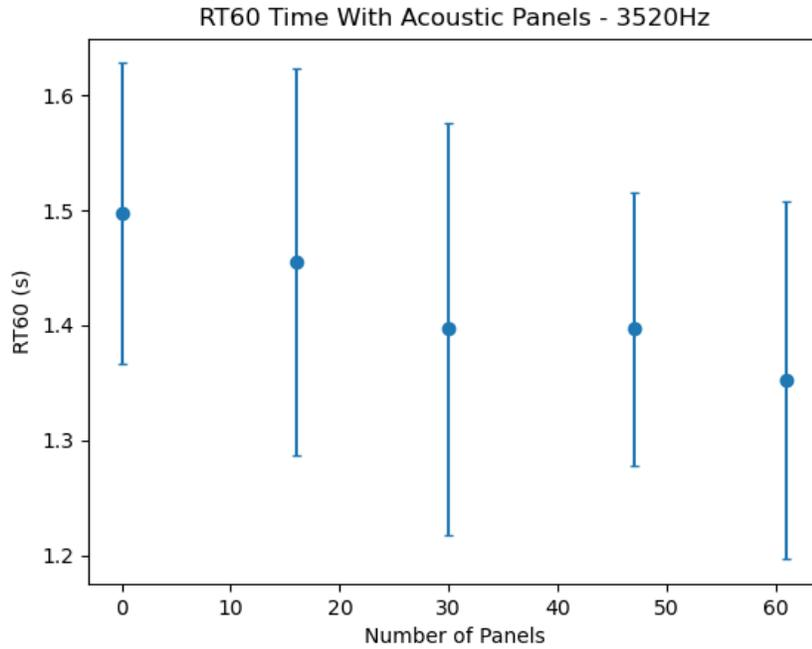
FIG. 16. The effect of acoustic paneling on decay time for 3520 - 7060 Hz. The RT60 time was extrapolated from 10 dB of decay.
