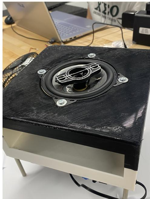
FIG. 5. The speaker is screwed into the top of the 3D printed box such that the cone is facing outward.
