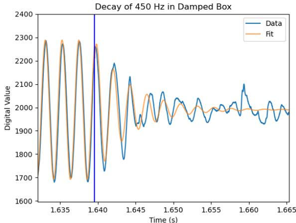
FIG. 7. The decay of a 450 Hz tone in the acoustic panel box. Here the blue line denotes where the tone was switched off. The calculated RT60 time is  $0.032 \pm 0.001$  seconds.
