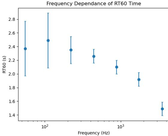
FIG. 11. The frequency dependence across octave ranges from 55 Hz to 7040 Hz. The locations of the points correspond to the lower end of their frequency band, and the frequency is in a logarithmic scale for ease of viewing. 440 - 1720 Hz were measured over 30 dB of decay, while other frequency bands were measured over 10 dB of decay.
