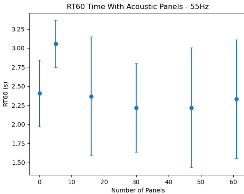
FIG. 17. The effect of acoustic paneling on decay time for 55 - 110 Hz. The RT60 time was extrapolated from 10 dB of decay.
