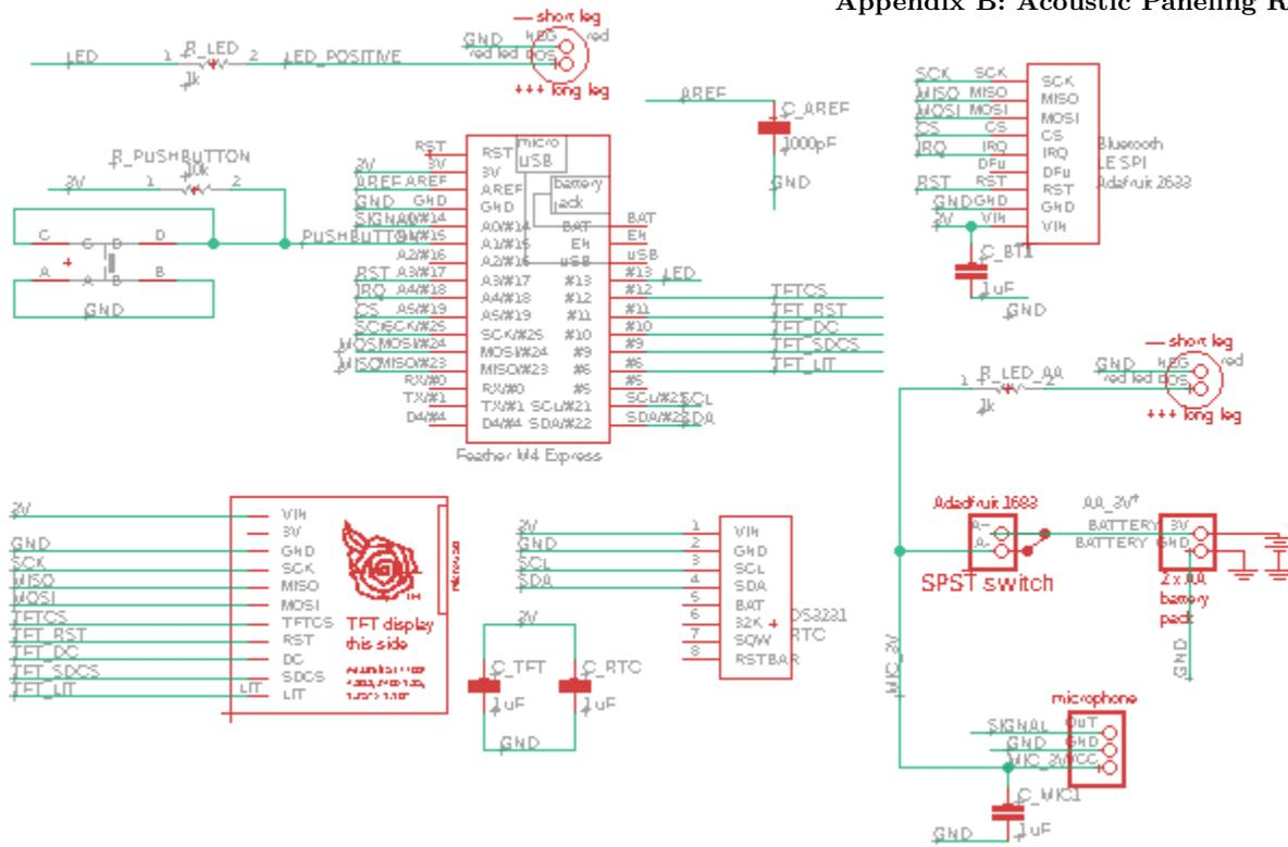
FIG. 15. Schematic of the microphone board.
