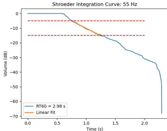
FIG. 10. The decay of the 55-110 Hz band of an impulse response in the studio. Here the red lines show the  $-5$  dB and  $-15$  dB levels between which the analysis takes place.
