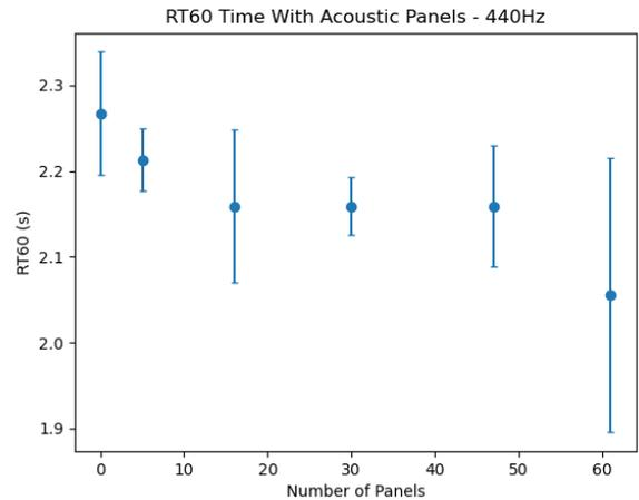
FIG. 13. The effect of acoustic paneling on decay time for 440 - 880 Hz. The RT60 time was extrapolated from 30 dB of decay.
