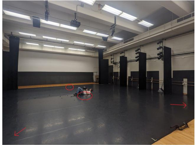
FIG. 12. The placement of 61 panels along the back and right wall of the studio. 25 were placed against the back concrete wall, 36 were covering the right concrete brick wall. Two of the microphone boards are located in the red circle in the middle of the room (near the sound source), one is in the red circle at the far end, and the other two are each in a corner outside of the picture denoted by the arrows.
