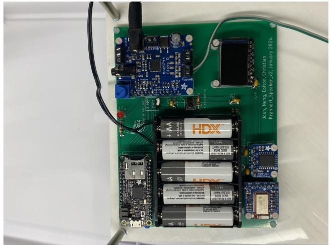
FIG. 4. The PCB of the speaker board is attached to a 3D printed box with four legs.
