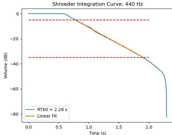
FIG. 9. The decay of the 440 - 880 Hz band of an impulse response in the studio. Here the red lines show the  $-5$  dB and  $-35$  dB levels between which the analysis takes place.
