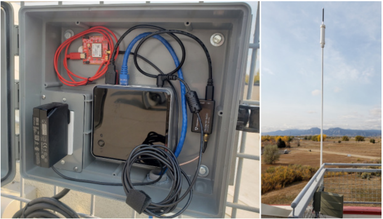
Figure 6: The SparkFun RTK Base Station complete with an NTRIP internet connection and a 915MHz RF connection
