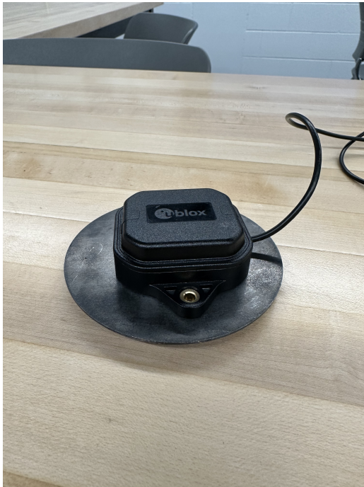
(a) ANN-MB-00 GNSS multiband antenna. Note the steel grounding plate. This adds approximately 0.4211 lbs to the system
