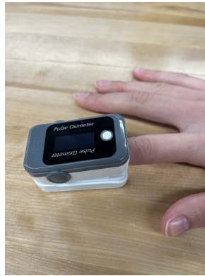
Figure 8: This figure shows a commercial pulse oximeter. This design uses a clamp over the finger to measure the pulse and blood oxygenation levels of a patient.
