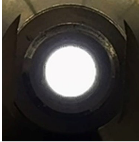
Fig. 11. Photograph of the mixed light produced by mixing CRGBV LEDs in the theoretical ratio calculated for white light. The result appears white in practice, confirming the effectiveness of our theory and modeling.
