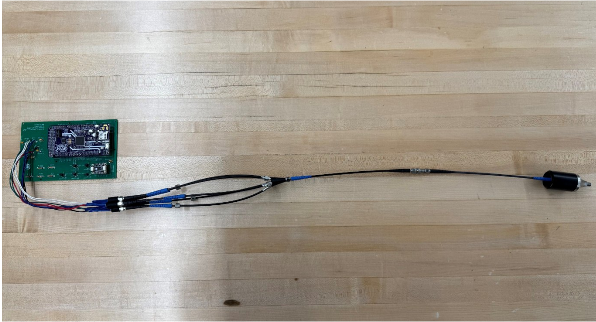
Fig. 7. The mix system. From left to right: PCB board with integrated LEDs; 3D printed LED-to-fiber adapters; optical fibers; 3D printed light mixing tube; another segment of optical fibers; and the final tube.
