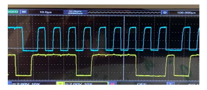
Play around with the "cursor" function to measure the clock speed. I find, with my setup, that the MEGA 2560 generates a clock pulse every  $10~\mu s$ , corresponding to a 100~kHz clocking rate.
