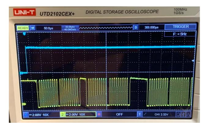
Now move your channel 1 signal to the "EXT TRIG" connector on the scope, and use a third probe so that the clock signal is on channel 1 and the data (SDI) line on channel 2. You should see something like this:
