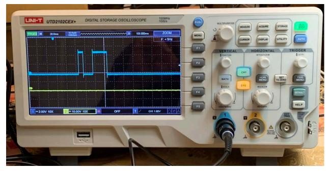
In the first, the scope trace is generated automatically at regular intervals even though nothing interesting is coming down the scope probe cable. In the second, the scope has triggered its trace in response to detecting a rising edge on channel 1.
