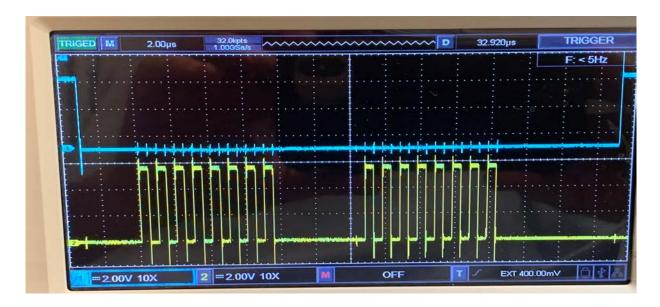
Note that the CS line is "active LOW": clock pulses are present when CS is LOW, not HIGH. Fool around with the cursor function to determine the clock speed... you should find that there's a clock pulse every microsecond, which is a factor of ten faster than the I2C clock.
