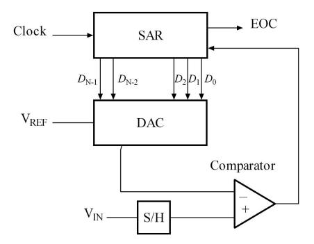
A successive-approximation ADC is a type of analog-to-digital converter that converts a continuous analog waveform into a discrete digital representation using a binary search through all possible quantization levels before finally converging upon a digital output for each conversion.
