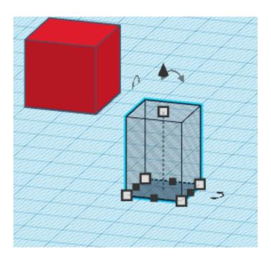
Select both objects and click on the "Align" tool. Align the horizontal centers, but leave the vertical unchanged.
