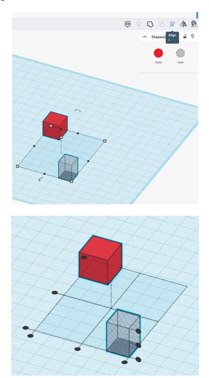
Note that I've set the red shape's color mode to "Transparent" in the following post-alignment image. The bottom faces of both the red box and the hole are at z = 0.
