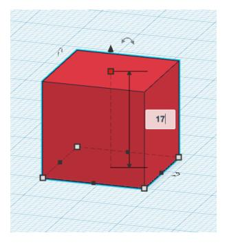
Now drag a cube-shaped "hole" onto the workplane. Set its width and depth to 14 mm but leave its height as 20 mm.
