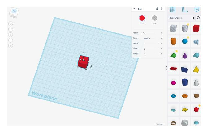
Now set the lengths of the cube's sides to 18 mm from the default of 20 mm.
