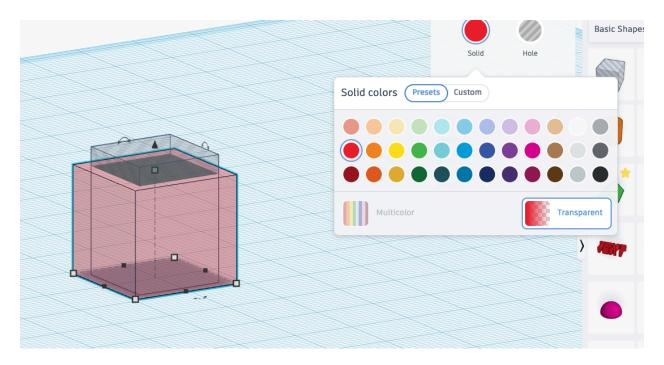
Now select only the hole and move it up 2 mm. On a Mac you can do this by holding down the command key and using the up arrow cursor. Perhaps with Windows you'd use ctrl instead of command?
