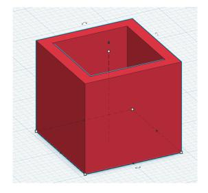
Now use the text basic shape to put your initials into the bottom of the box. Make the letters about 4 mm high so they extend above the floor of the box by 2 mm.
