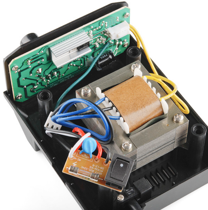
The insides of a soldering iron base
