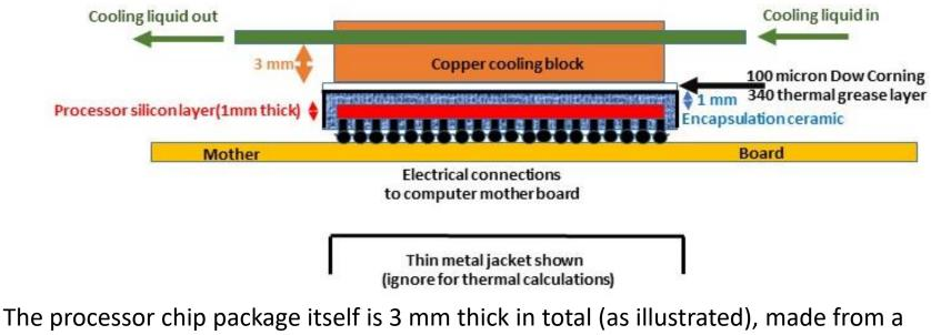
1 mm-thick active silicon layer centrally-sandwiched with 1 mm of ceramic encapsulant above & below it. The ceramic fill has a thermal conductivity of 200 Wm<sup>-1</sup>.K<sup>-1</sup>.
