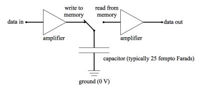
bit value and typical capacitor voltages:  $1 = 1.5 \ V$   $0 = 0 \ V$
