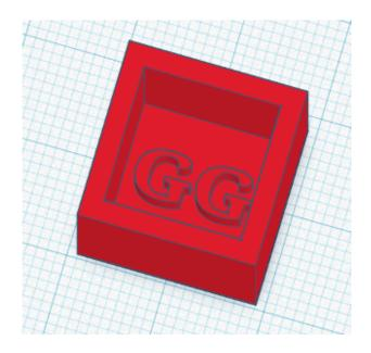
Now make the lid from a 1 mm thick square that's 18 mm on a side, and a 2mm thick square that's 13.5 mm on a side. (This'll give us a little bit of clearance.) have the bottoms of both squares set to z = 0. Put your initials on the lid, then group the lid components.
