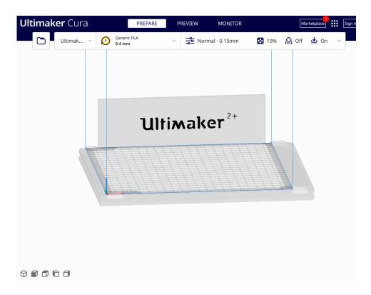
Drop the STL file from Tinkercad onto the Cura window. Click "slice" then save the gcode file to disk, then a microSD card.
