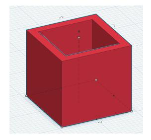
Now use the text basic shape to put your initials into the bottom of the box. Make the letters about 4 mm high so they extend above the floor of the box by 2 mm.
