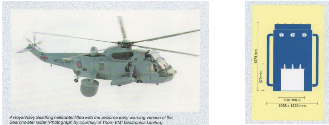
Fig. 2.2: Other examples: cooling an airborne military radar transmitter, cooling a transformer (traditionally using sulfur hexafluoride SF_6 ; GWP_{20y} of around 23000 \cdot CO_2 )
