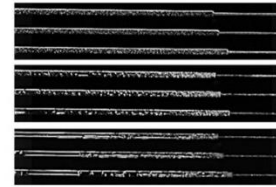
Fig. 7. Boiling CO 2 in micro-channels: upper to lower: 15 °C, 5 °C, -25 °C.
