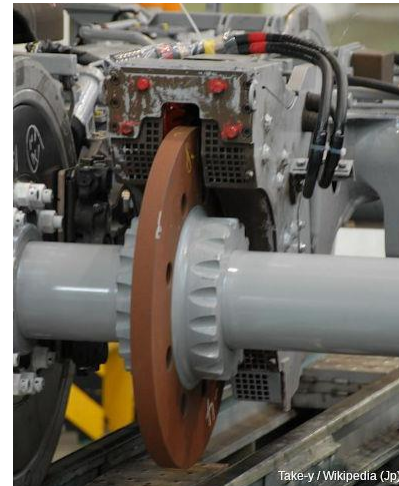
circular eddy-current brake from the Shinkansen 700 train
