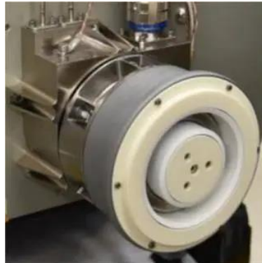
NGHT-1X Engineering Model Hall-Effect Thruster. Credits: Northrop Grumman
