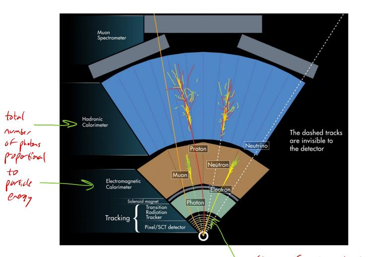
Strips of silicon: church particles deposit small anomes of everys in each pixel, can leave tracks Entire detector is immersed in - myneth field (out of the page in inner region): measure momentum and choose by curvature radius R = 3 m x <u>P\_L [Gev]</u> (4 1B1[T] If we know E and p => know m, particle ID
