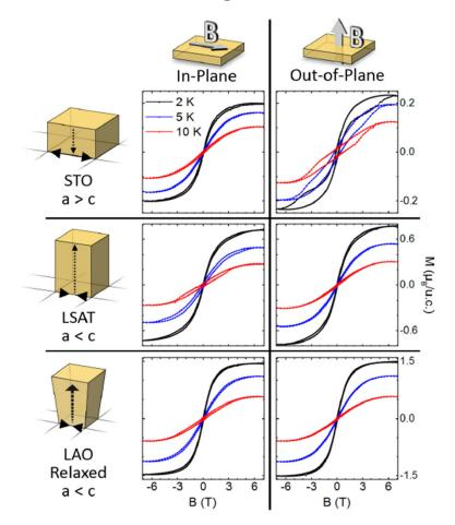
Different substrates induce different lattice strain. It would be interesting to see how different strains affect T5BO.
