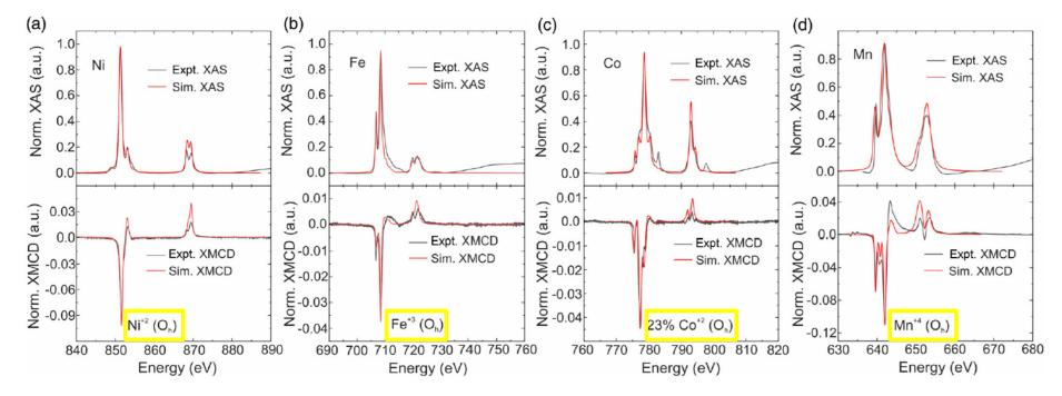
XAS and XMCD allow to determine the valencies of the elements Bonds involving Fe and Cr are known to support antiferromagnetism Bonds involving Mn4+ - O - Co2+ and Mn4+ - O - Ni2+ are known to support ferromagnetism T5BO is ferromagnetic
