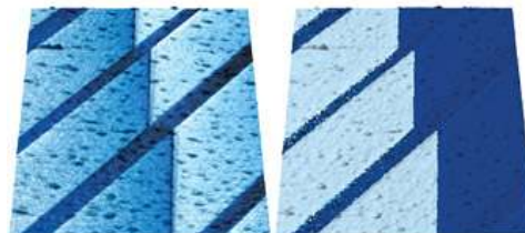
Figure 7.2.: PFM amplitude overlaid on AFM topography (left) and PFM phase overlaid on topography (right) on (100) oriented BaTiO 3 single crystal (from Cstech Crystals). The amplitude and phase image show 90° and 180° domain walls in BaTiO 3 . 10µm scan courtesy of V. R. Aravind, K. Seal, S. Kalinin, ORNL, and V. Gopalan, Pennsylvania State University.
