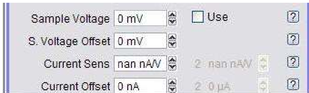
Figure 2.2.: These controls, found on the DoIV panel, control the bias to the sample while the sample is imaging.
