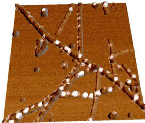
Figure 6.2.: Insulin Fibrils imaged in water. Phase signal overlaid onto topography. The “white” regions in the image are from the phase channel and correspond to higher energy dissipation. 1 \mu\text{m} scan.
