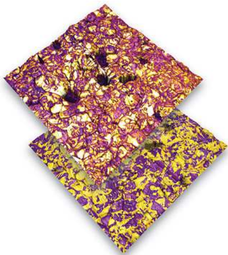
Figure 7.1.: PFM amplitude channel overlaid on AFM height (top) and phase image overlaid on height (bottom) of lead zirconium titanate (PZT), 20µm scan.
