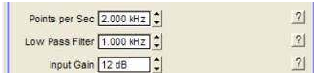
Figure 2.7.: [Filtering] You can set the digital filter to as low as needed. below 50Hz artifacts may appear. Be sure your filter is set to at least twice the frequency of your drive wave. note that complex wave forms (non sinusoidal) require much higher bandwidths to drive and acquire.
