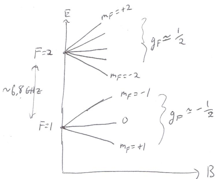
At high fields, where high means  $\Delta E_{\text{zeeman}} \sim \mu_B B_z \gg \Delta E_{\text{HF}}$ ,
