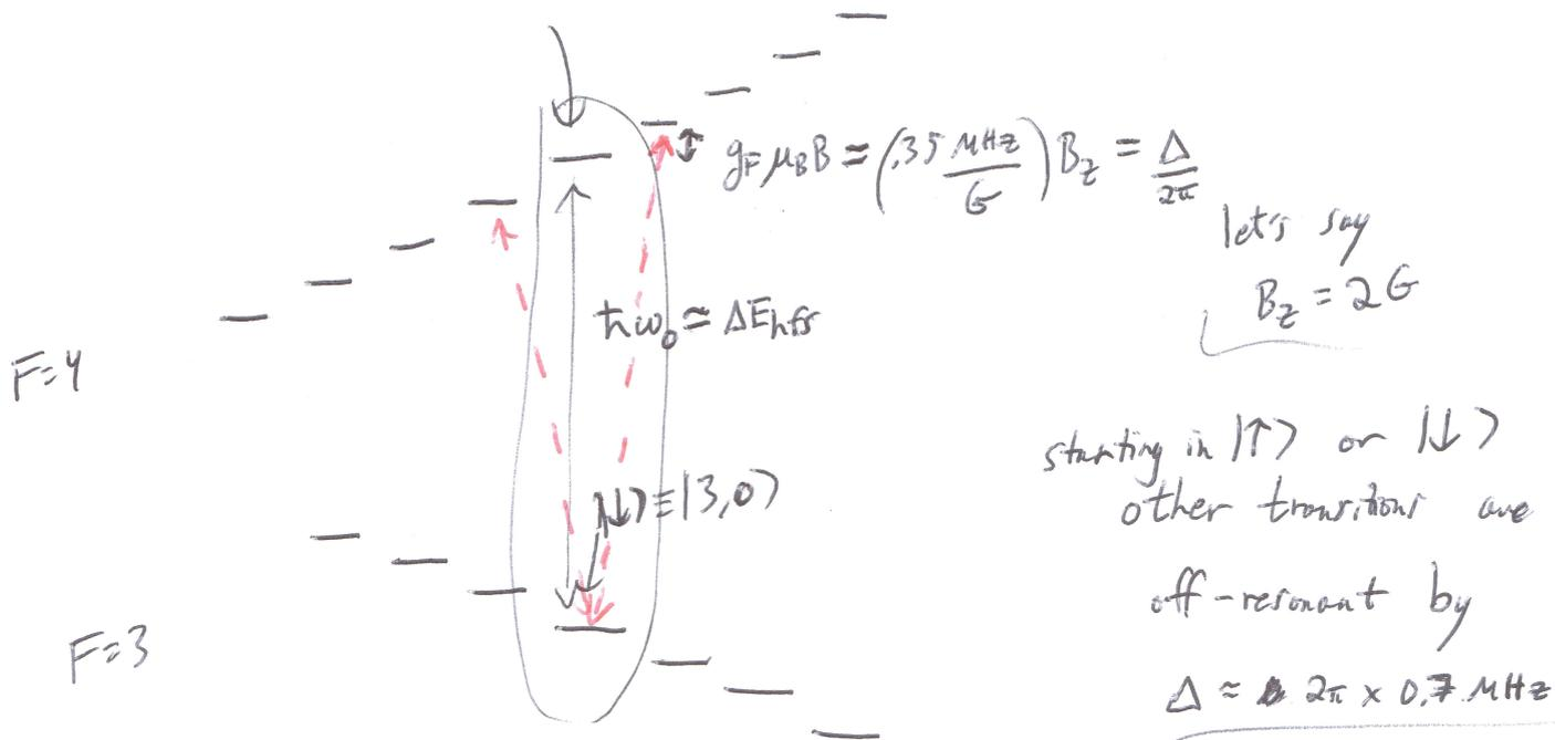
To avoid off resonant excitations, want corresponding  $P_{\text{other}}(t_{\pi})$  to be very small (where "other" refers to states w/ dipole-allowed transitions, like  $|4, \pm 1\rangle$ ).
