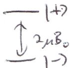
$$H = -\mu \tilde{\sigma}_z B_0 - \mu B_1 \tilde{\sigma}_x \cos(\omega t + \varphi)$$
