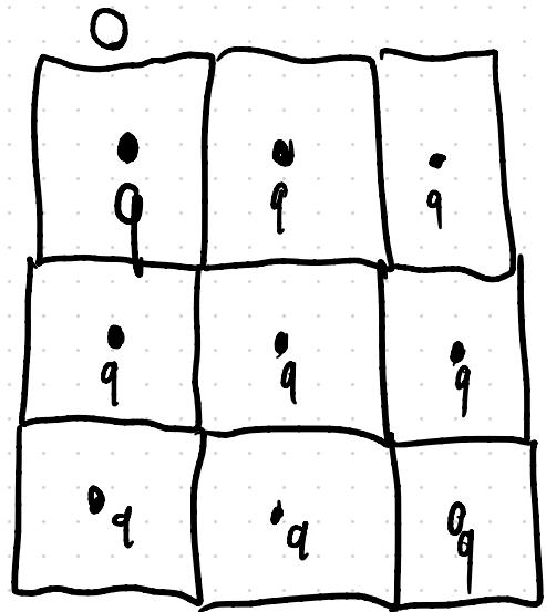
translations symmetry: identical atom at  $\vec{q} + \vec{R}$  for  $\vec{q} \parallel$  Bravais lattice vectors  $\vec{R}$
