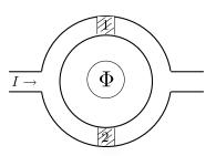
$$\Delta \phi_{AD} = \frac{e}{\hbar} \int_{D}^{A} \mathbf{A} d\mathbf{l}, \quad \Delta \phi_{CB} = \frac{e}{\hbar} \int_{B}^{C} \mathbf{A} d\mathbf{l}$$
