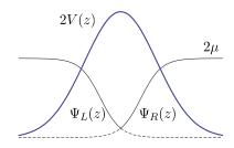
$$\Psi(z, \Delta\phi) = \Psi_R(z)e^{i\Delta\phi/2} + \Psi_L(z)e^{-i\Delta\phi/2}$$
