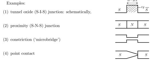
Josephson's original prediction for such links, originally made specifically for case (1) but often (not always!) valid for others, is 2 equations: If  $\Delta \phi$  denotes the phase difference of the GL OP (i.e., of the Cooper pairs) across the junction, then
